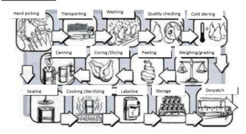
The flow chart shows the canning process for pears. There are fourteen stages in the procedure from when the fresh produce is picked to when the canned pears are distributed.
